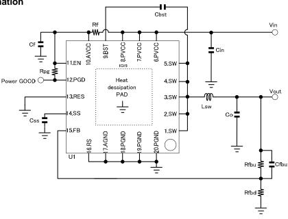
Figure 45. Recommended part circuit
