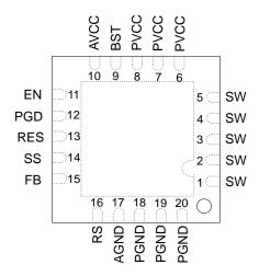
Figure 2. Pin Configuration
