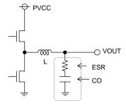
Figure 41. Output capacitor
