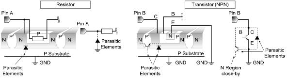
Figure 48. Example of monolithic IC structure
