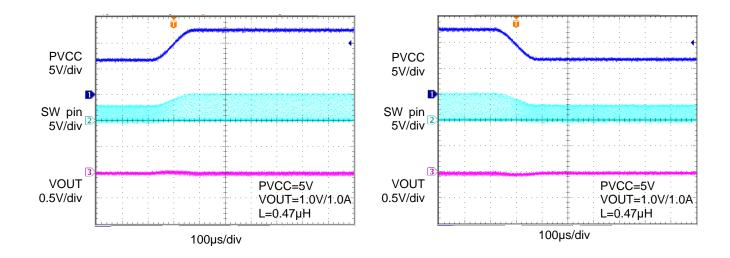
Figure 14. PVCC variation 2.9V to 5.5V
