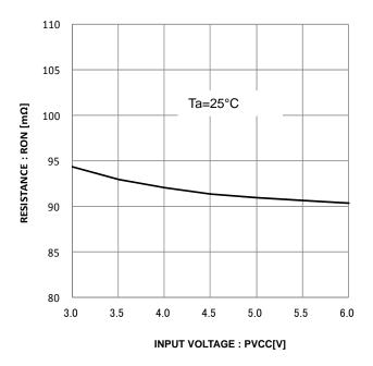
Figure 25. PowerGood MOSFET On-resistor
