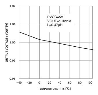
Figure 29. Output variation (ambient temperature)
