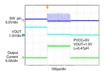
Figure 20. Output ground fault
