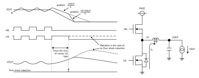
Figure 37. Over short reduction timing chart
