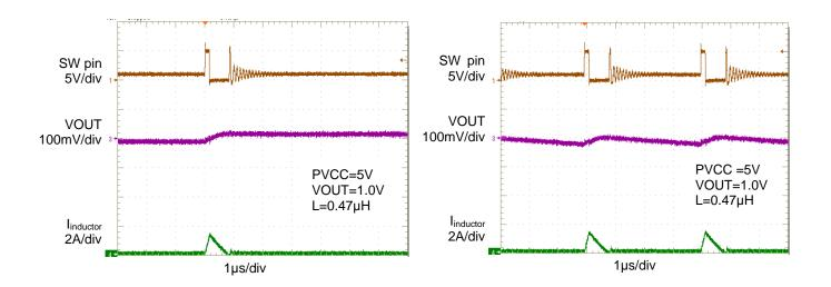
Figure 4. PFM operation, load 0mA
