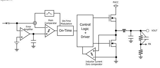
Figure 33. Constant on-time system block diagram
