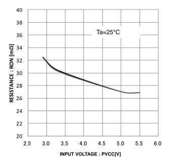
Figure 24. Power MOSFET On-resistor
