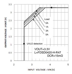
Figure 44. Output and input voltage difference limits
