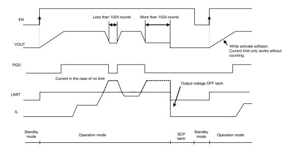
Figure 36. Over current protection/short-circuit protection function timing chart
