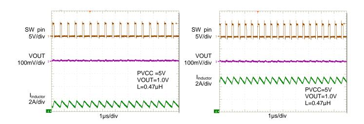
Figure 6. PWM operation, load 1000mA
