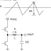
Figure 40. Output ripple current
