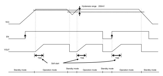
Figure 34. Soft Start, Shutdown, UVLO timing chart
