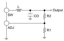
Figure 43. Output voltage setting resistor
