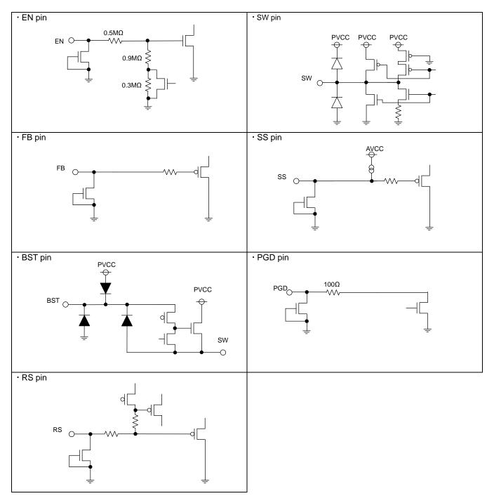
Figure 47. I/O equivalence circuit
