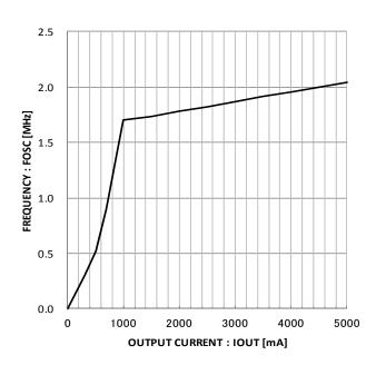
Figure 32. Frequency variation (Load regulation)
