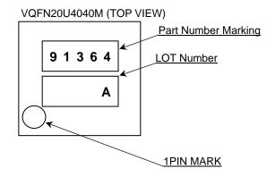
Physical Dimension, Tape and Reel Information Package Name VQFN20U4040M 4. 0±0. 1 1PIN MARK 15) □ 0. 05 C 0 R0.20 2.  $6 \pm 0$ . 1 UUUU20  $4\pm 0.05$ ci. 10 0 1 1 15 1. 0 0.  $25^{+0.05}_{-0.07}$ 0. 5 PKG: VQFN20U4040M Drawing No. EX375-5001 (UNIT: mm) <Tape and Reel information> Tape Embossed carrier tape Quantity 2500pcs The direction is the 1pin of product is at the upper left when you hold reel on the left hand and you pull out the tape on the right hand of feed Direction of feed 1pin
