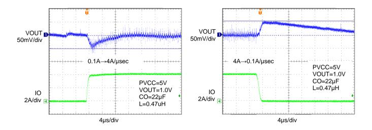
Figure 8. 0.1A to 4A Load transient response
