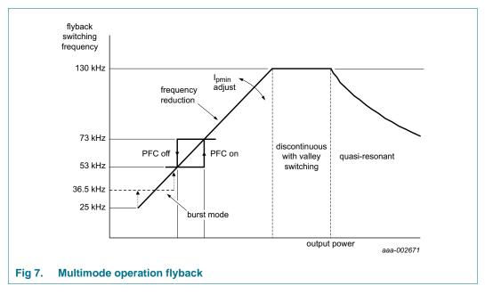
At high output power the converter switches to quasi-resonant mode. The next converter stroke starts after demagnetization of the transformer and detection of the valley. In quasi-resonant mode, switching losses are minimized. This minimization is achieved by the converter only switching on when the voltage across the external MOSFET is at its minimum (see Section 7.3.2).
