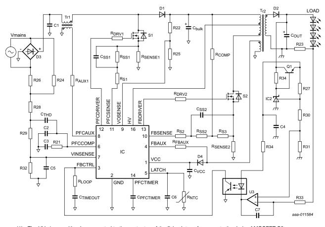
(1) The HV pin can either be connected to the center tap of the flyback transformer or to the drain of MOSFET S2.
