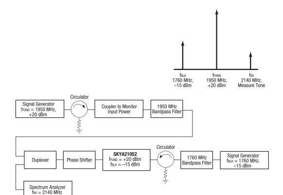
**Figure 4. Third Order Intermodulation Test Setup**
