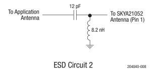
Figure 8. SKYA21052 Recommended ESD Protection Circuits
