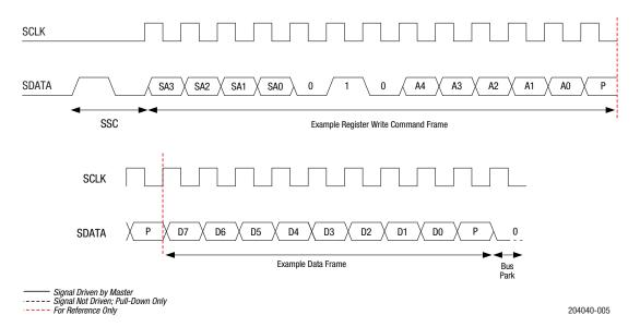
**Figure 5. Register Write Command Timing Diagram**
