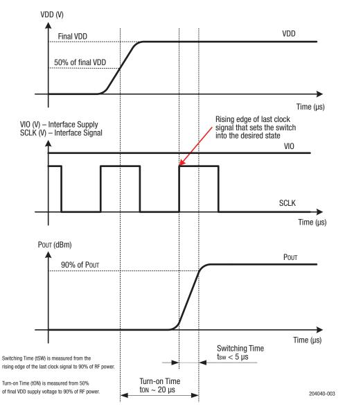
Figure 3. SKYA21052 Timing Diagram
