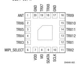
Figure 2. SKYA21052 Pinout (Top View)
