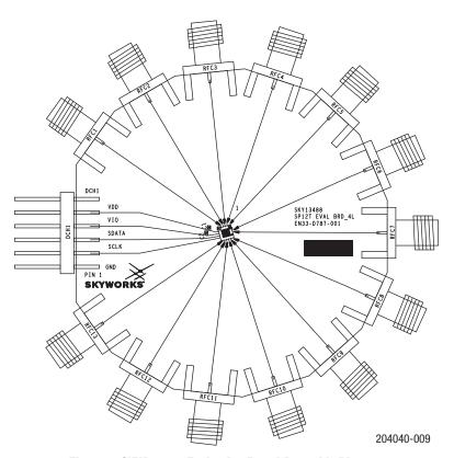
Figure 9. SKYA21052 Evaluation Board Assembly Diagram
