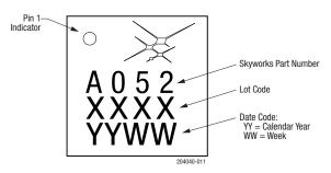
Figure 11. Typical Part Markings (Top View)
