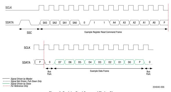
**Figure 6. Register Read Command Timing Diagram**
