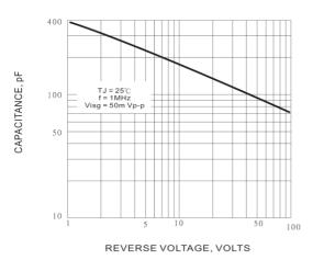
Fig.5 - TYPICAL JUNCTION CAPACITANCE PER ELEMENT
