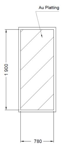
Chip thickness: 100µm +/- 10 µm All dimensions are in micrometers
