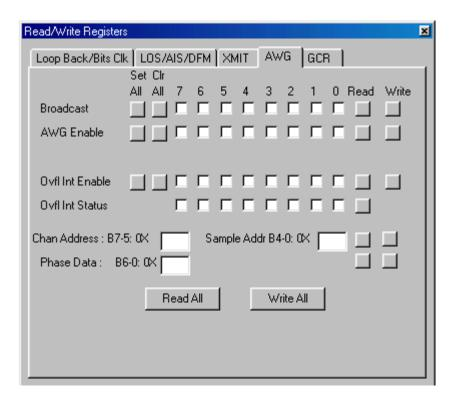
Figure 23. AWG Registers Screen
