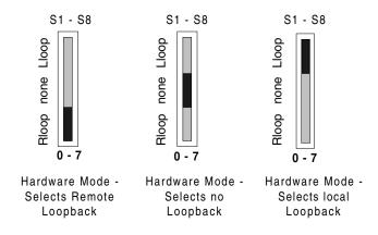
Figure 8. Loopback Mode Selection
