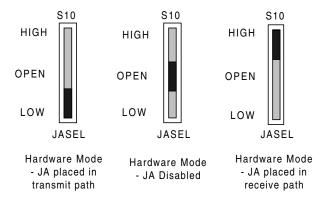
Figure 7. Jitter Attenuator Selection
