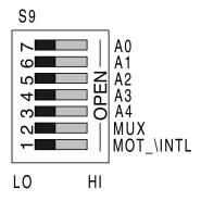
Hardware Mode - Enables HDB3/B8ZS coding & disables Channel 0 G.703 Bits Clock function
