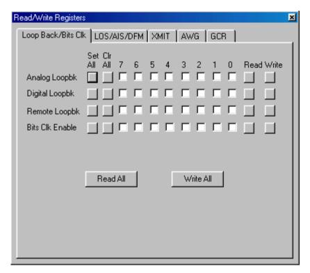
Figure 20. Loopback/G.703 Bits Clock Selection Screen
