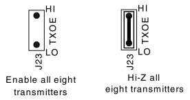
Figure 5. Transmitter Enable Selection
