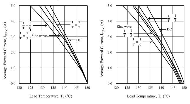
Figure 3-6  $I_{F(AV)} - T_L (V_R = 0 V)$
