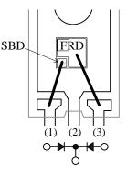
Figure 6-3 Internal structure of FMKS series
