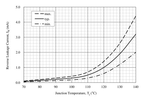
Figure 3-1 Temperature dependent of Reverse Leakage Current, I<sub>R</sub> (SBD)
