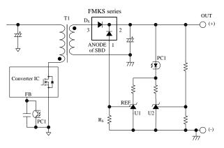
Figure 6-5 Reference temperature detection circuit with FMKS series.
