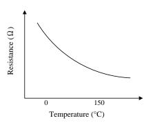
Figure 6-2 Reference characteristics of NTC thermistor
