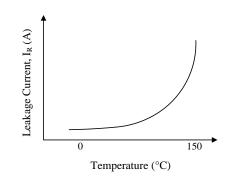
Figure 6-4 Reference temperature characteristics of SBD leakage current
