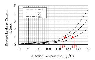
Figure 6-6 Temperature detection range at  $I_R = 1.0 \text{mA}$
