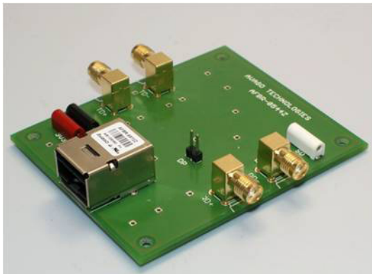
Figure 1. Evaluation board for the AFBR-5972Z transceiver module
