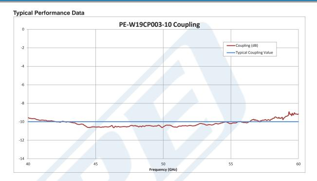
Click the following link (or enter part number in "SEARCH" on website) to obtain additional part information including price, inventory and certifications: WR-19 10 dB Directional Waveguide Coupler With UG-383/U Flange and E-Plane Coupled Port From 40 GHz to 60 GHz U Band PE-W19CP003-10
