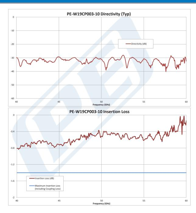
Click the following link (or enter part number in "SEARCH" on website) to obtain additional part information including price, inventory and certifications: WR-19 10 dB Directional Waveguide Coupler With UG-383/U Flange and E-Plane Coupled Port From 40 GHz to 60 GHz U Band PE-W19CP003-10
