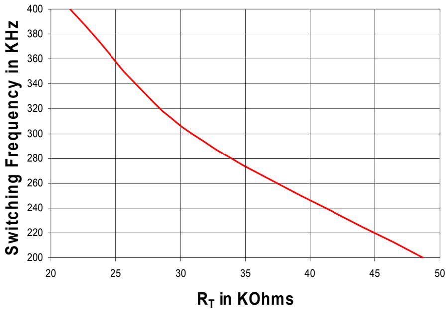
Fig. 2 : Per Channel Switching Frequency vs  $R_T$
