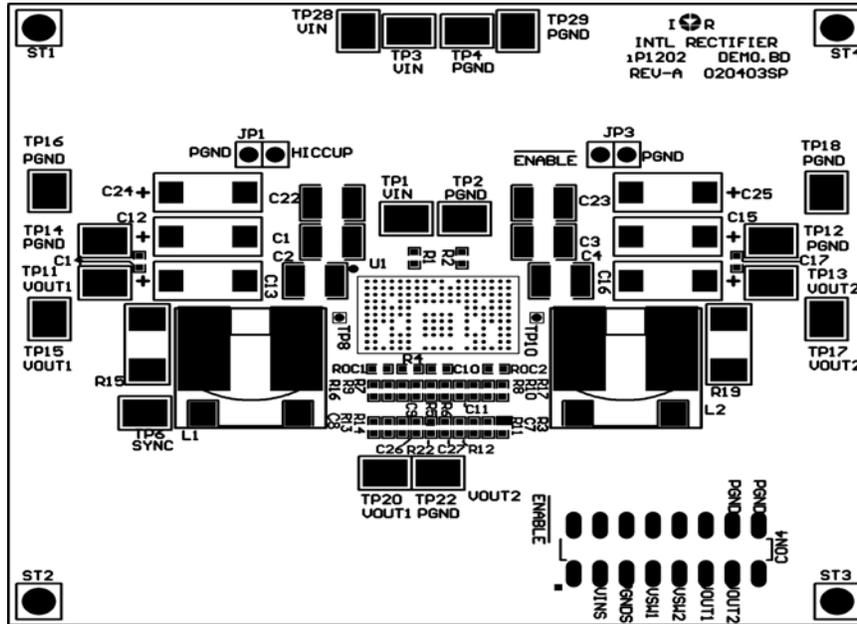
Fig. 5 - Component Placement (Top View) SideLayer
