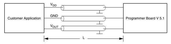
Fig. 3–1: Recommended wiring – schematic sketch
