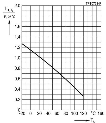
**Characteristics (typical) for  $T_{ref} = 130\text{ }^{\circ}\text{C}$**
