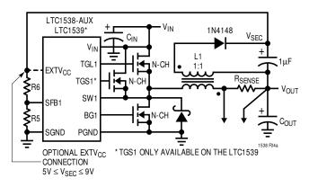
Figure 4a. Secondary Output Loop and EXTV<sub>CC</sub> Connection
