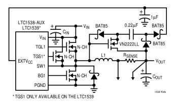
Figure 4b. Capacitive Charge Pump for EXTV<sub>CC</sub>
