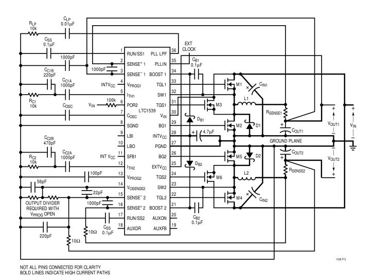
Figure 13. LTC1539 Physical Layout Diagram
