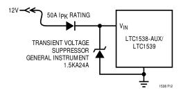
Figure 12. Automotive Application Protection
