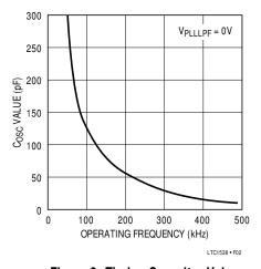
Figure 2. Timing Capacitor Value
