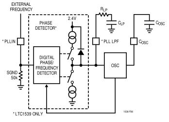
Figure 8. Phase-Locked Loop Block Diagram
