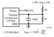
Figure 5b. LTC1538-AUX/LTC1539 Adjustable Applications
