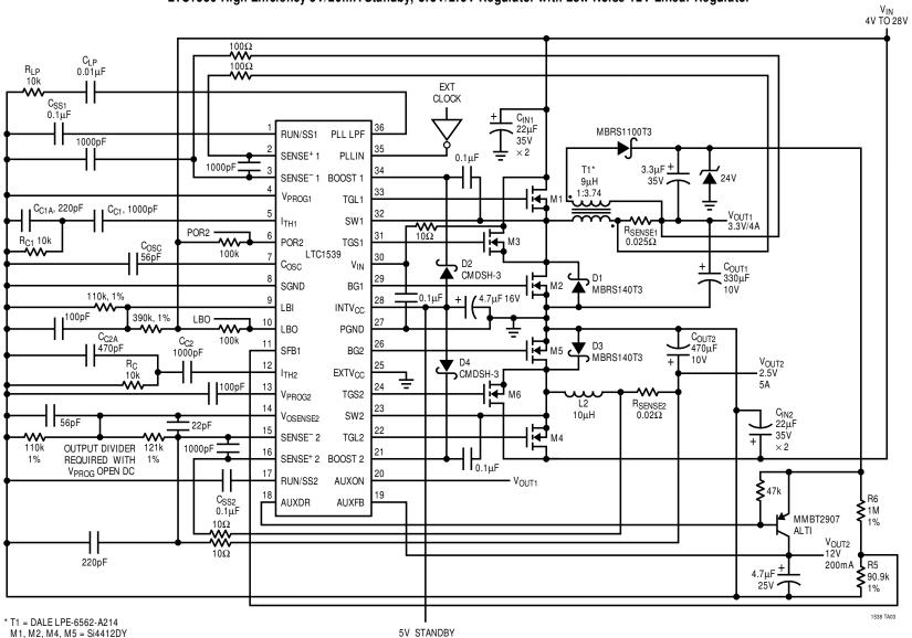
M1, M2, M4, M5 = Si4412DY M3, M6 = IRLML2803 L2 = SUMIDA CDRH127-100MC INPUT CAPACITORS ARE AVX-TPS SERIES OUTPUT CAPACITORS ARE AVX-TPSV LEVEL II SERIES
