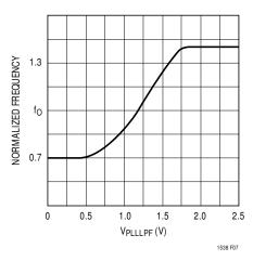
Figure 7. Operating Frequency vs V<sub>PLLLPF</sub>
