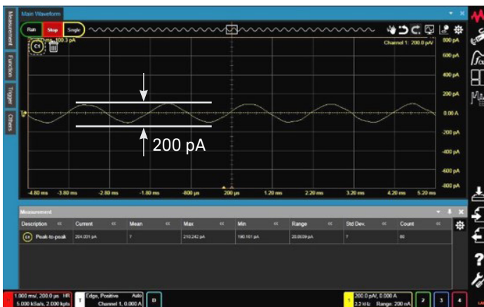
Figure 4. Very-low current measurement example: 200 pA peak-to-peak current waveform.
