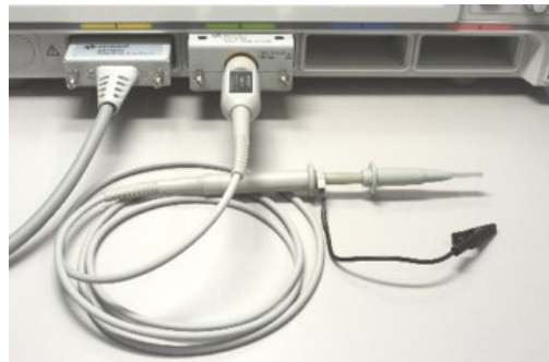
Figure 7. The CX3300 series can also measure and view voltage waveforms using a passive probe, so that you can view the dynamic power waveforms as well as current waveforms.
