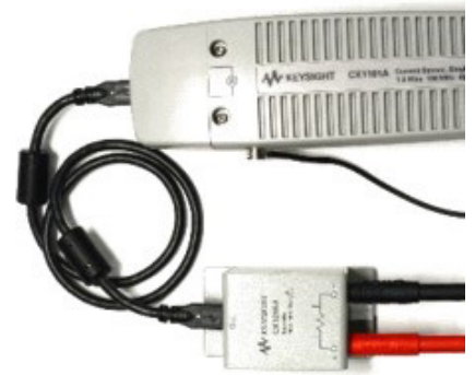
Figure 32. CX1206A and CX1101A. Even when you evaluate low power devices, you may occasionally need to measure higher current at more than 1 A. The CX1206A sensor head with expander enables CX1101A current sensor to measure from 3 mA to 10 A current waveforms based on the ESL (Effective Series Inductance) reduced shunt resistor technology.
