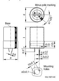
Snap-in terminals, length (6.3 + 1/-1.4) mm. Also available in a shorter version with a length of (4.5 - 1.4) mm. PET insulation cap is positioned under the insulation sleeve. Safety vent on the base or on the case wall.
