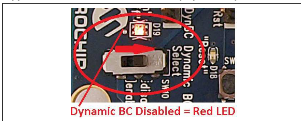
FIGURE 2-11: DYNAMIC BATTERY CHARGE SELECT DISABLED
