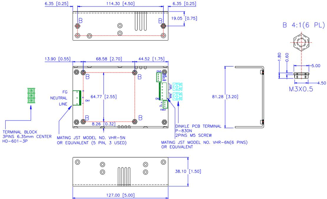
E Type (Enclosed with Rear Side built-in Fan): 6.5(L) x 3.2(W) x 1.6(H) inches; Weight: 650g.
