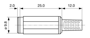
Cable diameter max. 4.0 mm
