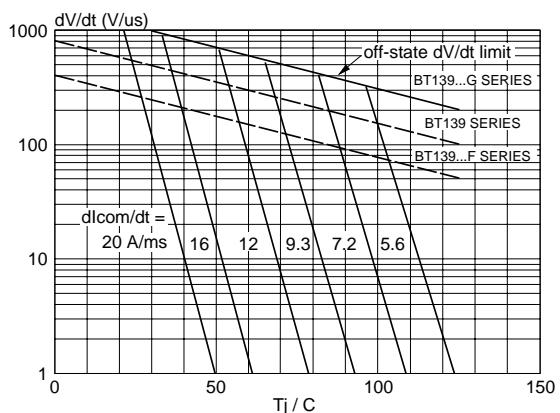
*Fig.12. Typical commutation  $dV/dt$  versus junction temperature, parameter commutation  $dl/dt$ . The triac should commutate when the  $dV/dt$  is below the value on the appropriate curve for pre-commutation  $dl/dt$ .*
