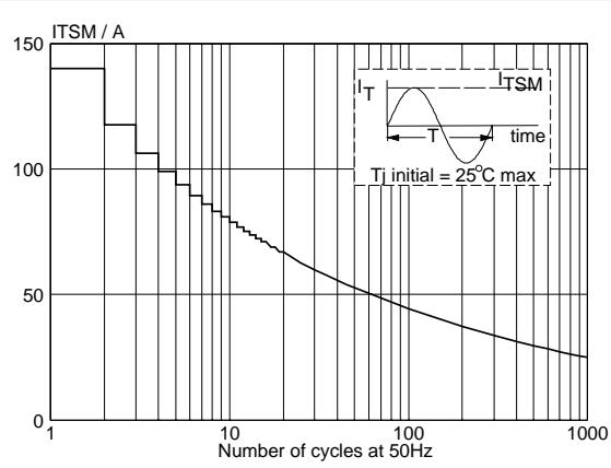
*Fig.3. Maximum permissible non-repetitive peak on-state current  $I_{TSM}$ , versus number of cycles, for sinusoidal currents,  $f = 50\text{ Hz}$ .*
