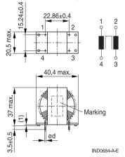
Tolerances to ISO 2768-C unless otherwise noted. Dimensions in mm.
