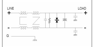
The 1135 series is designed to provide filtering for DC systems operating in very noisy environments.
