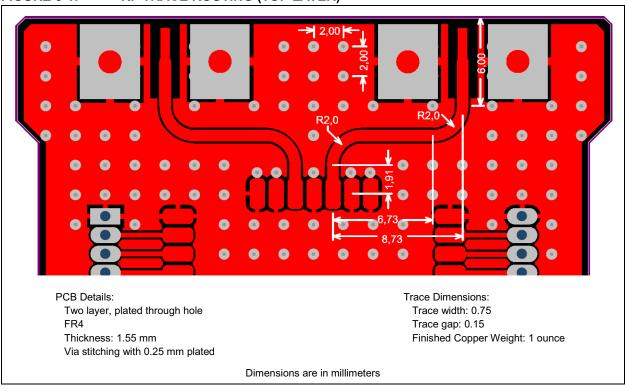
FIGURE 5-2: RF TRACE ROUTING (BOTTOM LAYER)
