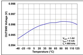
**FIGURE 2-6:** OUTSNS Voltage vs. Temperature.
