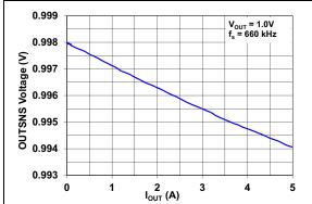
**FIGURE 2-19:** Load Regulation: OUTSNS Voltage vs. I<sub>OUT</sub>.
