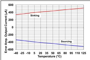
**FIGURE 2-12:** Error Amplifier Output Current vs. Temperature.
