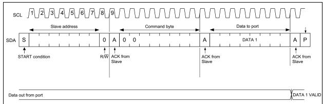
FIGURE 8-3: Single Write Timing Diagram.
