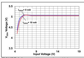
FIGURE 2-2: V<sub>DDA</sub> vs. Input Voltage.
