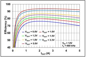
FIGURE 2-16: Efficiency vs. Load Current.
