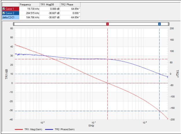
FIGURE 2-40: Voltage Loop Gain Bode Plot,  $V_{OUT}$ = 1.8V,  $f_{\rm S}$ = 570 kHz, L = 1.2 μH,  $C_{OUT}$ = 266 μF,  $R_{C1}$  = 2.55kΩ,  $C_{C1}$  = 10nF,  $C_{C2}$  = 47pF (see Section 7.7, Compensation Design).
