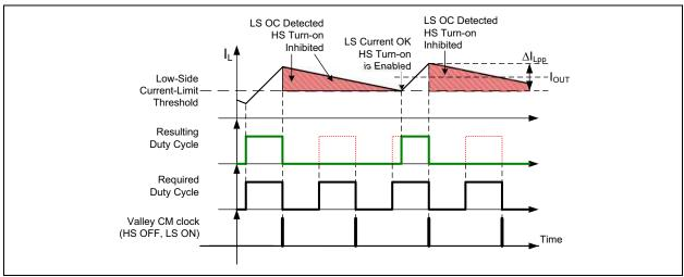
FIGURE 4-1: Low-Side Cycle-by-Cycle Current-Limit Action.
