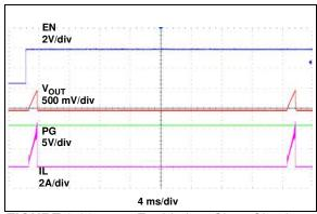
FIGURE 2-30: Enable into Short Circuit.
