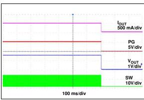
FIGURE 2-33: Thermal Shutdown Response.
