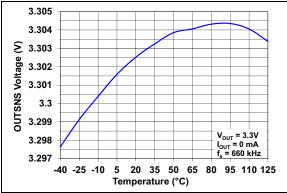
FIGURE 2-8: OUTSNS Voltage vs. Temperature.
