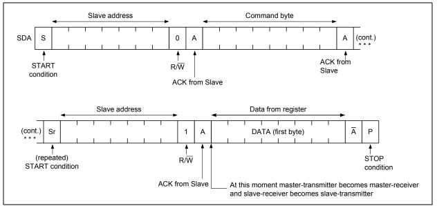
FIGURE 8-5: Single Read Timing Diagram.
