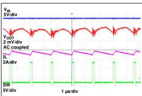
**FIGURE 2-36:** Switching Waveforms -  $f_S = 660 \text{ kHz}$ ,  $I_{OUT} = 5A$ .
