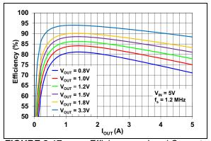
FIGURE 2-17: Efficiency vs. Load Current.
