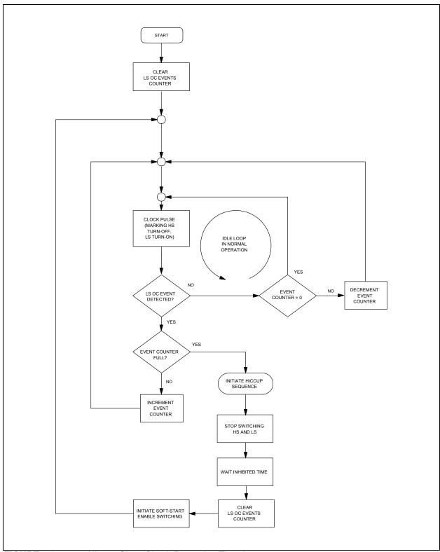
FIGURE 4-2: Hiccup Short-Circuit Protection Flowchart.
