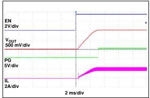
**FIGURE 2-25:** EN Turn-on,  $R_{LOAD} = 0.3\Omega$ .
