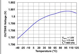
FIGURE 2-7: OUTSNS Voltage vs. Temperature.
