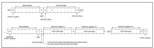
FIGURE 8-6: Block Read Timing Diagram.
