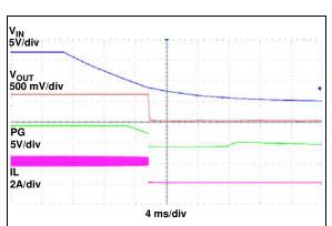
FIGURE 2-24:  $V_{IN}$  Turn-off (EN =  $V_{DDA}$ ),  $R_{LOAD} = 0.3\Omega$ .
