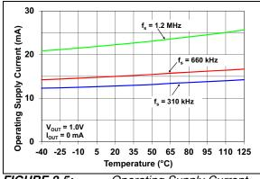
FIGURE 2-5: Operating Supply Current vs. Temperature, Switching.
