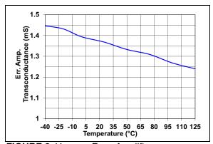
FIGURE 2-11: Error Amplifier Transconductance vs. Temperature.
