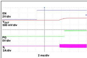
**FIGURE 2-28:** EN Turn-on into pre-biased output  $(V_{pre-bias} = 0.8V)$ .
