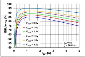
FIGURE 2-15: Efficiency vs. Load Current.
