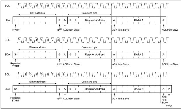
FIGURE 8-4: Single Write with Repeated Start Timing Diagram.
