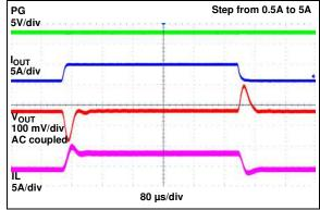
**FIGURE 2-38:** Load Transient Response with  $I_{LIM} = I_{LIM\_LS3}$ .
