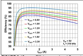
FIGURE 2-13: Efficiency vs. Load Current.
