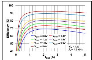
FIGURE 2-18: Efficiency vs. Load Current.
