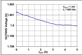
**FIGURE 2-20:** Load Regulation: OUTSNS Voltage vs. I<sub>OUT</sub>.
