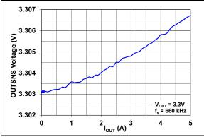
FIGURE 2-21: Load Regulation: OUTSNS Voltage vs. I<sub>OUT</sub>.
