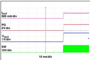
FIGURE 2-34: Recovery from Thermal Shutdown.
