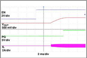
**FIGURE 2-27:** EN Turn-on into pre-biased output  $(V_{pre-bias} = 0.5V)$ .
