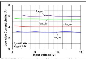
FIGURE 2-3: Low-Side Current Limits vs. Input Voltage.
