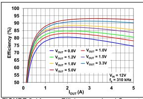
FIGURE 2-14: Efficiency vs. Load Current.
