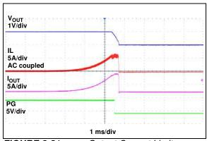
FIGURE 2-31: Output Current Limit Threshold.
