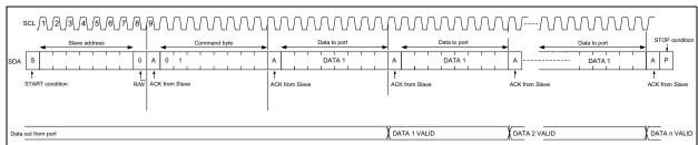
FIGURE 8-7: Block Write Timing Diagram.
