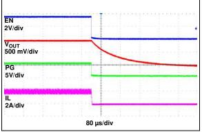
**FIGURE 2-26:** EN Turn-off,  $R_{LOAD} = 0.3\Omega$ .
