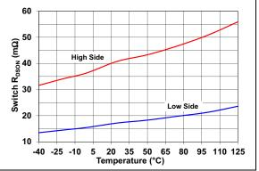
**FIGURE 2-10:**  $R_{DS(on)}$  vs. Temperature.
