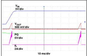
**FIGURE 2-29:** Power-up into Short Circuit,  $(EN = V_{DDA}, no \ ^2C \ programming, registers default values for 2Z version).$
