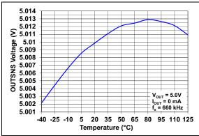
FIGURE 2-9: OUTSNS Voltage vs. Temperature.
