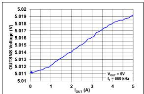
FIGURE 2-22: Load Regulation: OUTSNS Voltage vs. I<sub>OUT</sub>:
