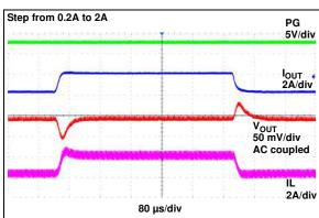
**FIGURE 2-37:** Load Transient Response with  $I_{LIM} = I_{LIM}$  LSO.
