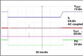
**FIGURE 2-32:** Hiccup Mode Short Circuit Current Limit Response.
