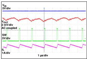
**FIGURE 2-35:** Switching Waveforms -  $f_S = 660 \text{ kHz}$ ,  $I_{OUT} = 0A$ .
