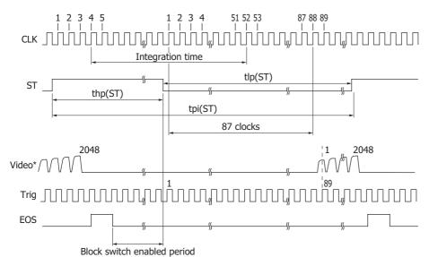
\* When reading from 1024 pixels, the Video signal is output from 513 to 1536 channels.
