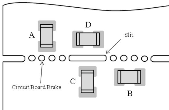
Stress strength according to the mounting position:
