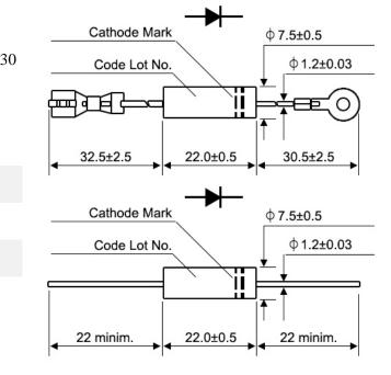
$V_{RM}=V_{RRM}$ , f=50Hz,  $T_{AMB}=100^{\circ}$ C Half sine voltage with f=50Hz applied,  $T_{AMB}=100^{\circ}$ C  $T_{AMB}=130\pm2^{\circ}$ C Solder trough temp.: 350±10°C, Dip Time: 3.5s ± 0.5s 120°C, 2 x 10<sup>5</sup>pa Between the center of the body and terminal (*See Fig. 1*) 1 min. between center of the body and terminal. (*Fig.1*) Force 10 N to the lead, bent it to pos. and neg. 90°
