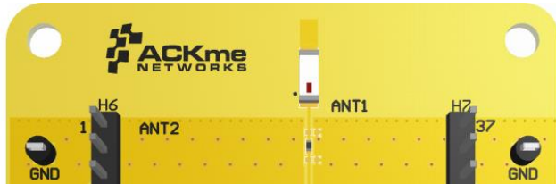
Figure 10 – Chip antenna layout example
