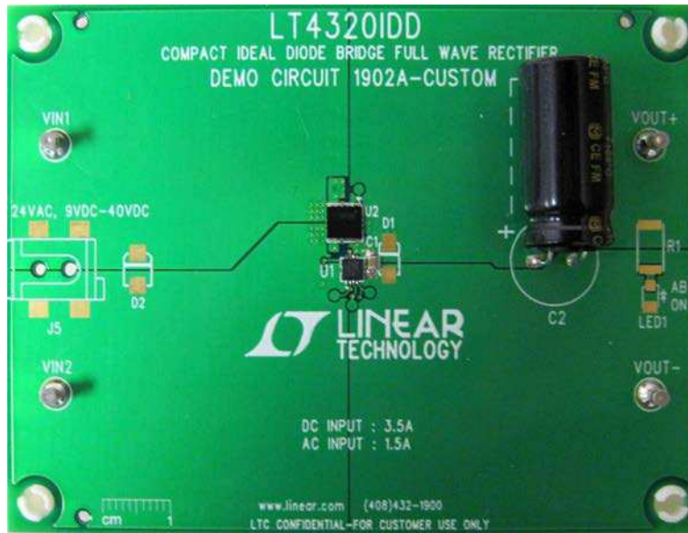
Figure 4. Demonstration Circuit 1902A Used in Figure 3 Thermograph
