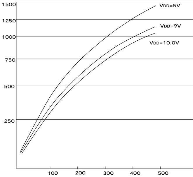
Figure 4.  $T_{ow}$  vs  $R_{BIAS}$ , k $\Omega$
