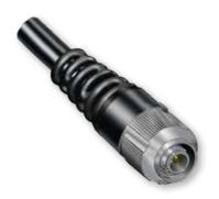
Harsh Environment Cordsets Overmolded Series 811 cordsets withstand abrasion and chemical exposure. Cable construction features silver coated stranded conductors with TFE insulation, tinned copper braid shield and extruded black polyurethane jacket. Choose single-ended pigtails or double-ended "back-to-back" cables. Semi-rigid polyamide overmold provides strain relief and environmental sealing.
