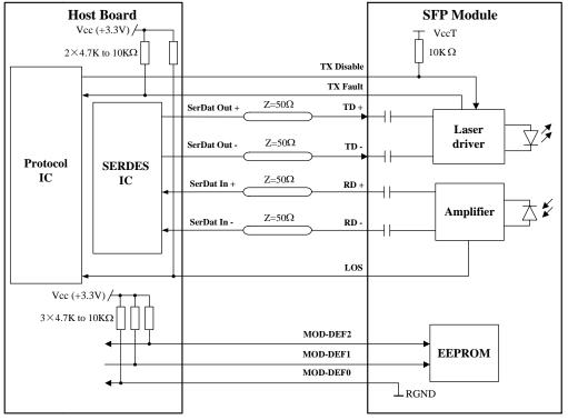
Figure 2, Recommended Interface Circuit
