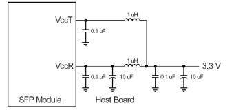
Figure 1, Recommended Host Board Power Supply Circuit
