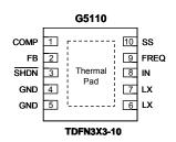
Note: Recommend connecting the Thermal Pad to the Ground or let it keep floating.
