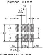
**Terminal Arrangement and Internal Connections** (Top View)
