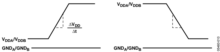
Figure 13. Transient Immunity Waveforms—Output Supplies
