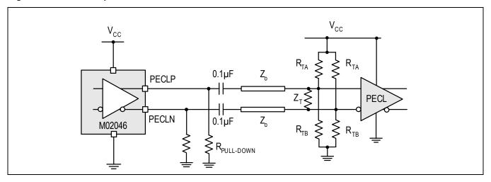
Figure 4-7. DC-Coupled PECL Termination
