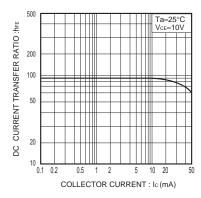
Fig.1 DC current gain vs. collector current
