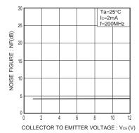
Fig.10 Noise factor vs. collector voltage
