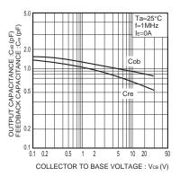
Fig.3 Capacitance vs. reverse bias voltage
