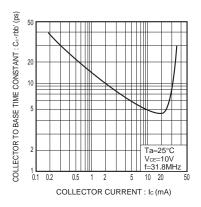
Fig.5 Collector to base time constance vs. collector current
