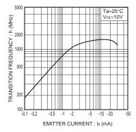
Fig.4 Gain bandwidth product vs. emitter current
