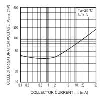
Fig.2 Collector-emitter saturation voltage vs. collector current
