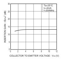
Fig.8 Insertion gain vs. collector voltage
