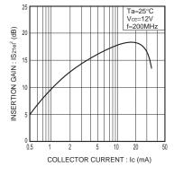
Fig.7 Insertion gain vs. collector current
