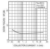
Fig.9 Noise factor vs. collector current
