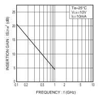
Fig.6 Insertion gain vs. frequency
