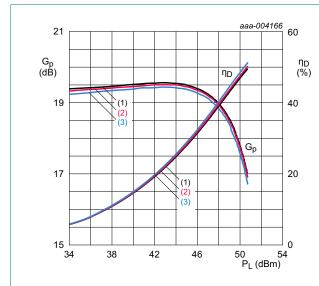
$V_{DS} = 30 \text{ V}; I_{Dq} = 1100 \text{ mA}.$
