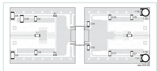
Printed-Circuit Board (PCB): Rogers RO4350;  $\epsilon_r$  = 3.5 F/m; thickness = 0.762 mm; thickness copper plating = 35  $\mu$ m.
