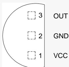
Figure 2. Pin Configuration of AP3700/A (Top View)
