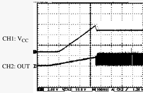
Figure 8. Start-up Sequence of  $V_{CC}$  and  $V_{OUT}$
