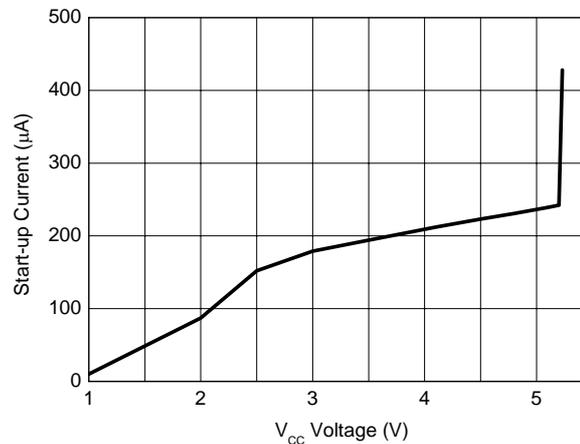
Figure 7. Start-up Current vs. V<sub>CC</sub> Voltage
