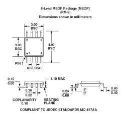
Figure 2. μSOIC-8 —Dimensions shown in millimeters
