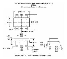
Figure 1. SOT23-6—Dimensions shown in millimeters
