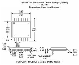
Figure 3. TSSOP-14 ---- Dimensions shown in millimeters
