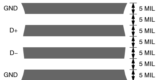
Figure 16. Arrangement of Signal Tracks
