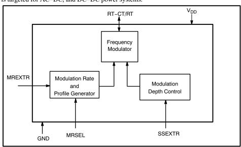
Figure 1. Block Diagram
