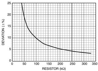
Figure 5. Deviation vs. SSEXTR (@ Switching Frequency = 1.6 MHz, MR = 25 kHz)
