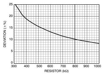
Figure 3. Deviation vs. SSEXTR (@ Switching Frequency = 280 kHz, MR = 25 kHz)
