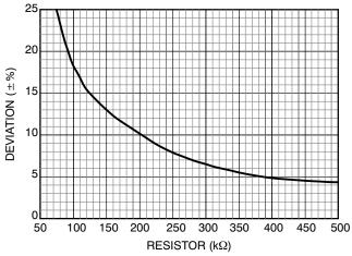
Figure 4. Deviation vs. SSEXTR (@ Switching Frequency = 1 MHz, MR = 25 kHz)
