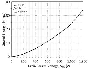
Figure 10: Output Capacitance Stored Energy
