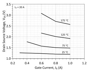
Figure 4: Drain-Source Voltage vs. Gate Current
