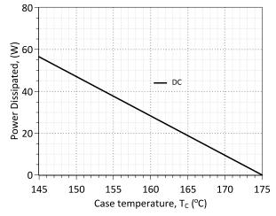
Figure 16: Power Derating Curve
