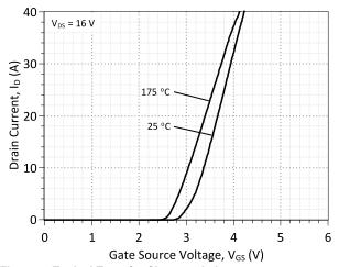
Figure 7: Typical Transfer Characteristics
