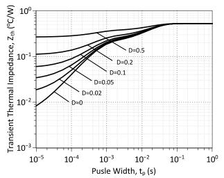
Figure 20: Transient Thermal Impedance
