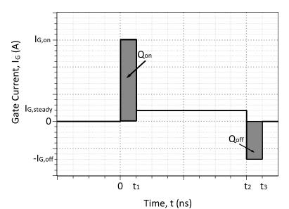
Figure 22: Idealized Gate Current Waveform
