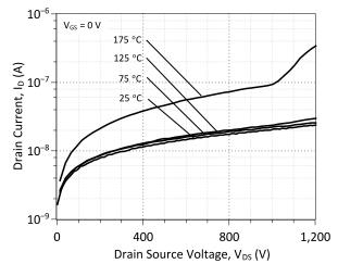
Figure 8: Typical Blocking Characteristics
