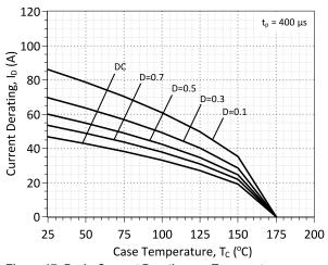
Figure 17: Drain Current Derating vs. Temperature
