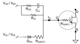
Figure 24: Primary gate drive circuit passive components with series gate resistance Schottky rectifier.
