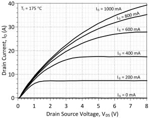
Figure 3: Typical Output Characteristics at 175 °C
