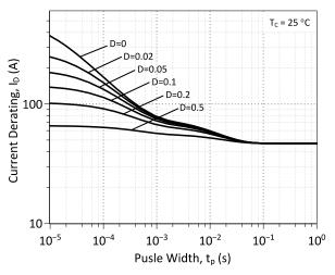
Figure 21: Drain Current Derating vs. Pulse Width
