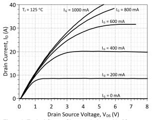
Figure 2: Typical Output Characteristics at 125 °C
