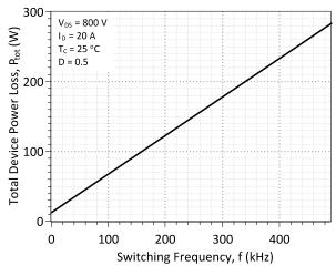
Figure 15: Typical Hard Switched Device Power Loss vs. Switching Frequency <sup>2</sup>
