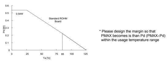
Figure 83. SSOP5 Power dissipation heat reduction characteristics (Reference)
