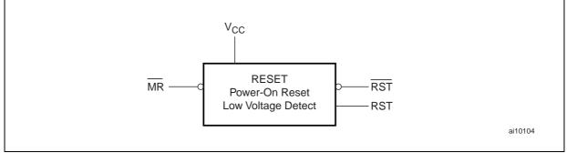
Note: V<sub>CC</sub> is the supply voltage, MR is the Manual Reset input. RST and RST are Reset outputs. Supervisor devices can have an active-Low output (RST), an active-High output (RST) or both.
