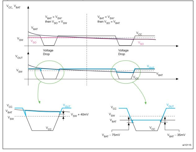
Figure 12. Switchover Waveforms with Hysteresis Details
