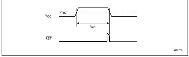
Note: 1. For the STM818, E<sub>CON</sub> is held Low, externally. The E<sub>CON</sub> state is latched half way through the t<sub>REC</sub> period, and the Freshness Seal function is enabled.
