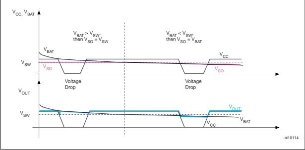
Note: The red line represents the switchover voltage ( $V_{SO}$ ). The blue line represents the battery switchover circuit output voltage ( $V_{OUT}$ ), which is switched to  $V_{CC}$ , or to  $V_{BAT}$  depending on the voltage magnitude.
