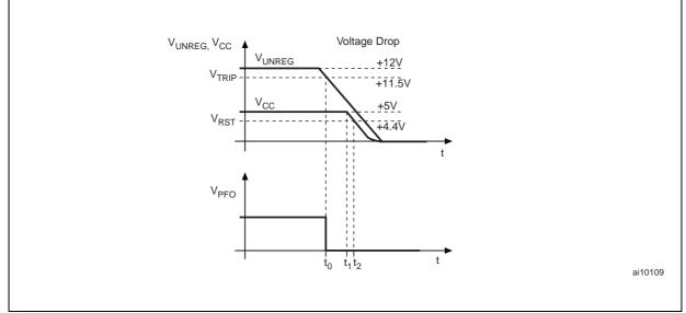
Note: At  $t_0$  the voltage drop is detected; at  $t_1$  V<sub>CC</sub> begins to fall; at  $t_2$  Reset is asserted and/or Write Protect occurs.
