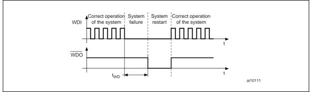
Note: 1. WDI signal frequencies greater then 50MHz (20ns period) will be filtered. 2. t<sub>WD</sub> is the Watchdog time-out period. See Table 7. for value.
