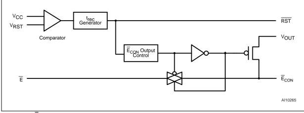
Figure 15. Chip Enable Gating Block Diagram
