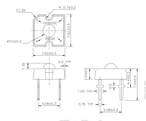
Note: Tolerances unless mentioned  $\pm 0.25$ mm. Unit = mm
