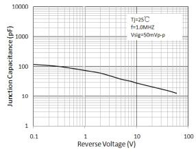
Figure 4. Typical Junction Capacitance
