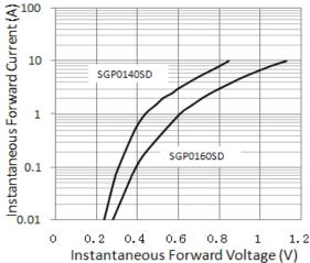
Figure 2. Typical Instantaneous Forward Characteristics
