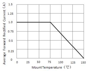
Figure 1. Forward Current Derating Curve
