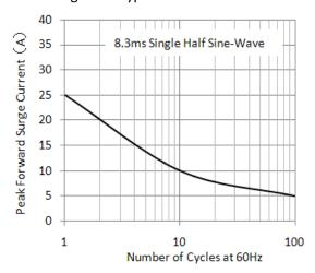
Figure 5.Maximum Non-Repetitive Peak Forward Surge Current
