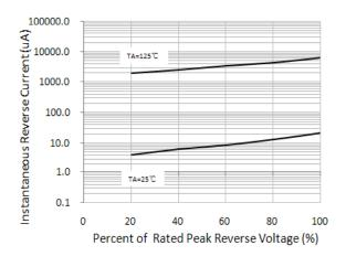
Figure 3. Typical Reverse Characteristics
