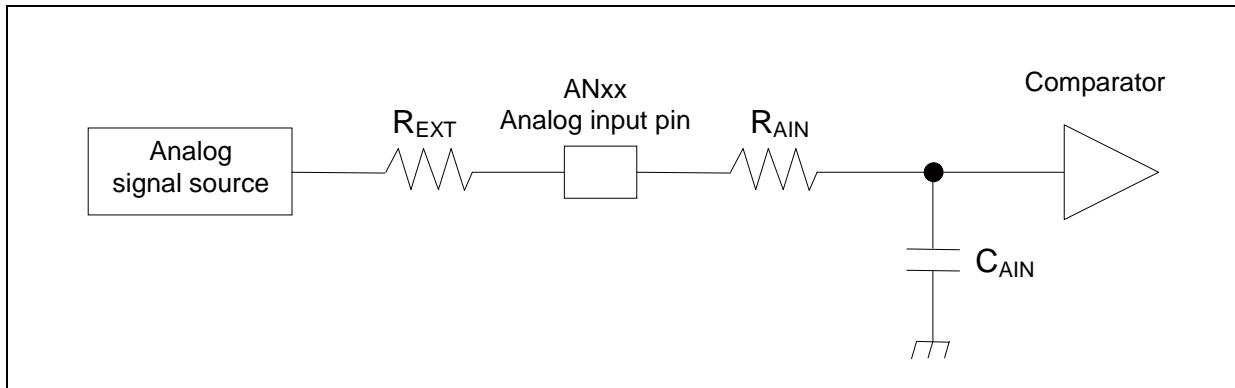
$$(Equation 1) t_S \geq (R_{AIN} + R_{EXT}) \times C_{AIN} \times 9$$
