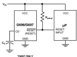
ICC may increased at high T<sub>A</sub>, Therefore, can not connect Resistors to VCC to prevent Icc abnormal behavior at high T<sub>A</sub>.
