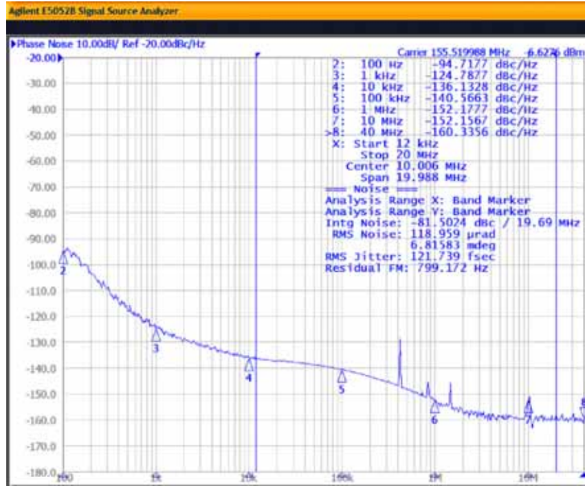
Figure 7. Input = 25 MHz; Output = 155.52 MHz, 2.5 V LVDS
