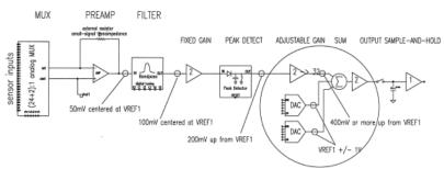
The sum is done in the gain stage, so the signal won't roil internally
